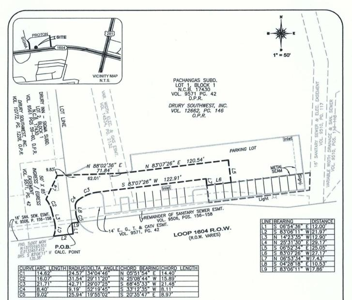
BEARING AND COORDINATES ARE BASED ON LAMBERT GRID, TEXAS STATE PLANE COORDINATES, SOUTH CENTRAL ZONE NAD 83/93; COORDINATES SHOWN HEREON HAVE AN APPLIED SURFACE SCALE FACTOR OF 1.00017
