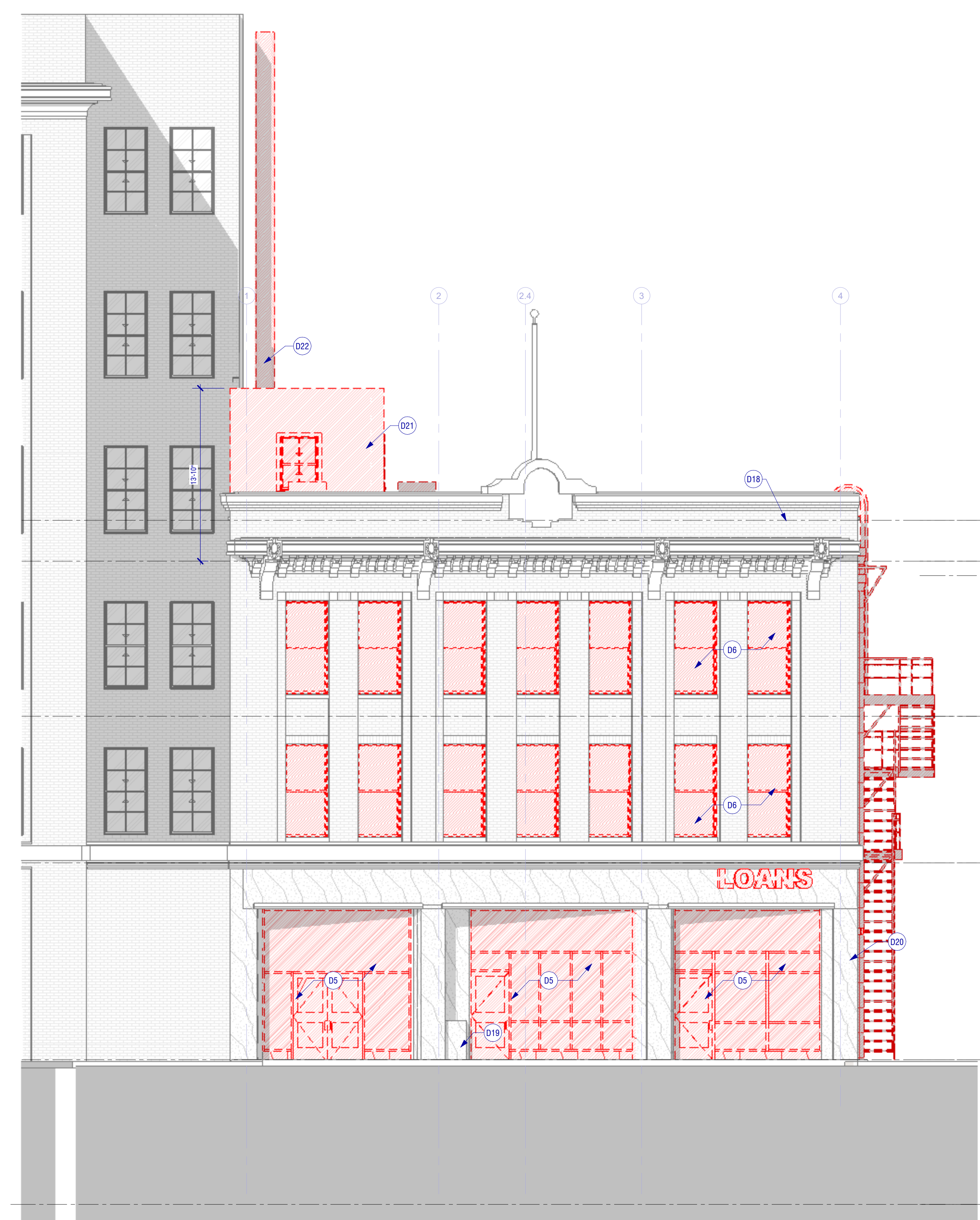
2 DEMO SOUTH ELEVATION 3/16" = 1'-0"
