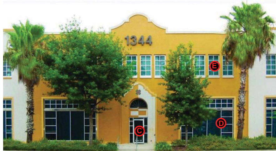
D EXHIBIT D NON-HISTORIC ALUMINUM STOREFRONT W/ TINTED GLASS ON EXISTING OPENING
