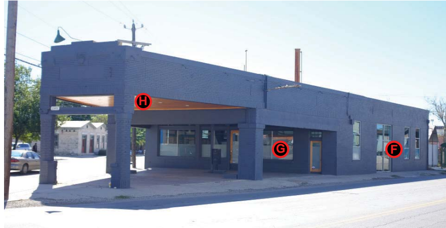
G EXHIBIT G NON-HISTORIC ALUMINUM STOREFRONT W/ FROSTED FILM ON EXISTING STOREFRONT OPENING
