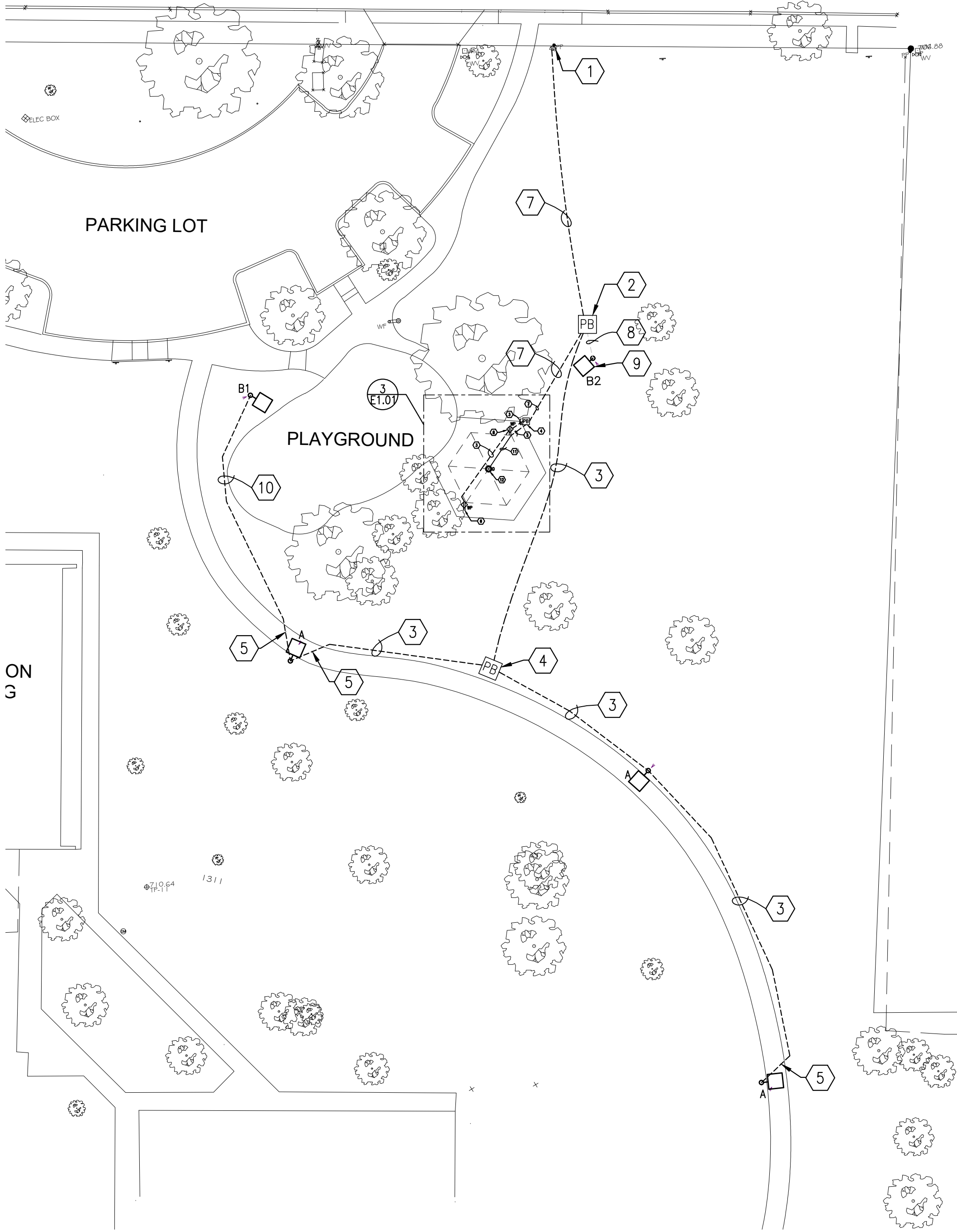
2 ELECTRICAL SITE PLAN - PLAYGROUND SCALE: 1" = 30'
