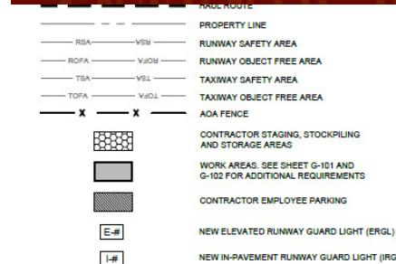
1. ALL AOA PAVEMENT SURFACES SHALL BE OPEN FOR AIRPORT OPERATIONS AT ALL TIMES UNLESS OTHERWISE DESIGNATED AND APPROVED BY THE RPR FOR SPECIFIC CONSTRUCTION WORK PERIODS. THE AOA CONSISTS OF THE AREA INSIDE THE PERIMETER SECURITY FENCE.
