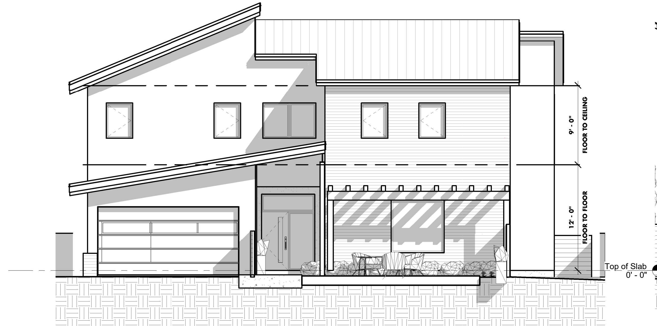
1 Standalone Residence-West Elevation 3/16" = 1'-0"
