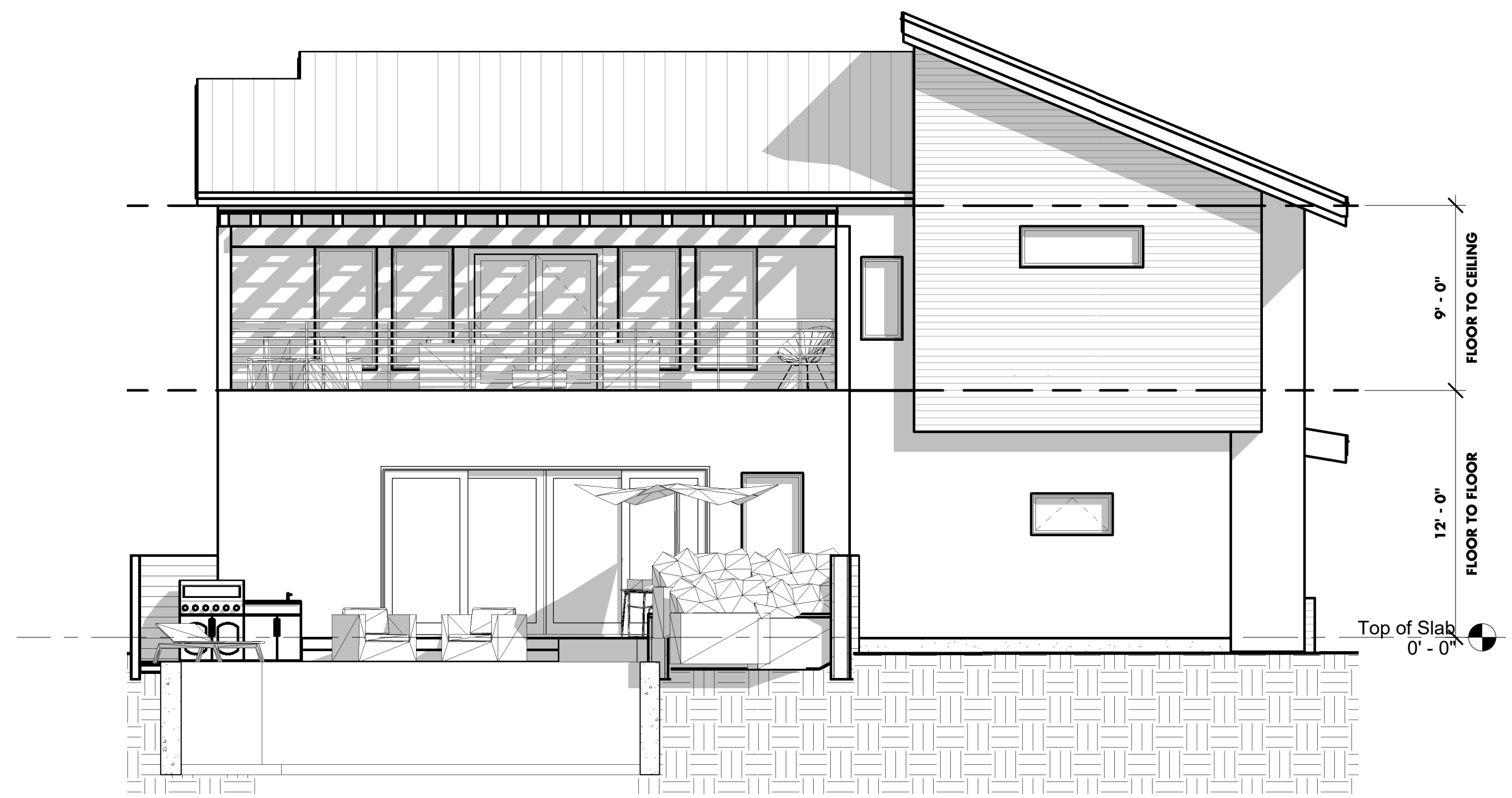
3 Standalone Residence-East Elevation 3/16" = 1'-0"
