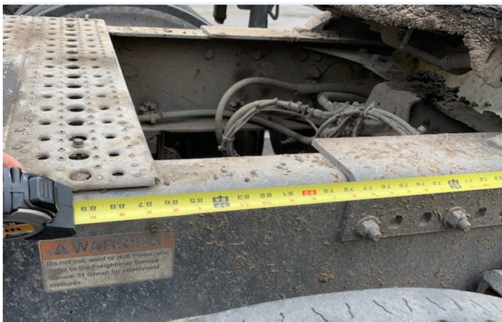
Photo 3: Measurement of chassis rail and fifth wheel adjusted length.
