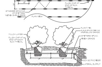
3 1/2" X 1/2" SUB-SURFACE DRIP IRRIGATION DETAIL
