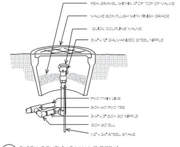
5 QUICK COUPLING VALVE DETAIL
