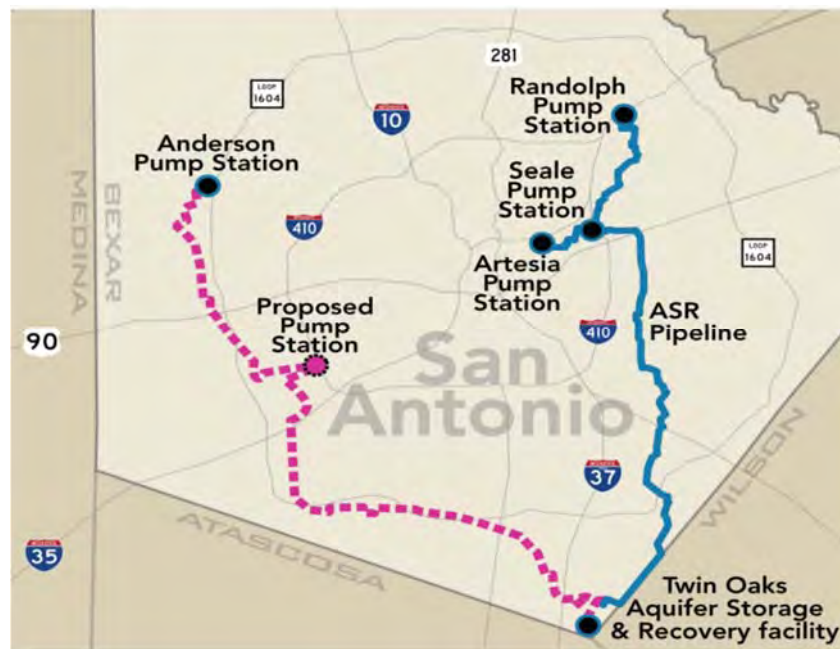
Figure 25: Proposed new pipeline that will bring water from southern Bexar County to the eastern and western sides of its service area, to enhance flexibility 42 .
