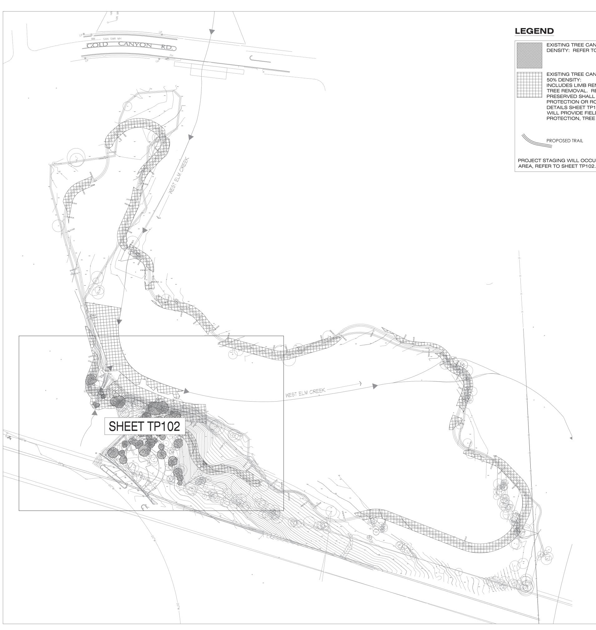
EXISTING TREE CANOPY TO BE REMOVED AT 100% DENSITY: REFER TO SHEET TP102 EXISTING TREE CANOPY TO BE REMOVED AT UP TO INCLUDES LIMB REMOVAL AND/OR COMPLETE TREE REMOVAL. REMAINING TREES TO BE PRESERVED SHALL BE PROTECTED BY TREE TRUNK PROTECTION OR ROOT PROTECTION FENCING PER DETAILS SHEET TP103. LANDSCAPE ARCHITECT WILL PROVIDE FIELD DIRECTION FOR TREE PROTECTION, TREE PRUNING, AND TREE REMOVAL. PROPOSED TRAIL PROJECT STAGING WILL OCCUR AT THE PROPOSED PARKING
