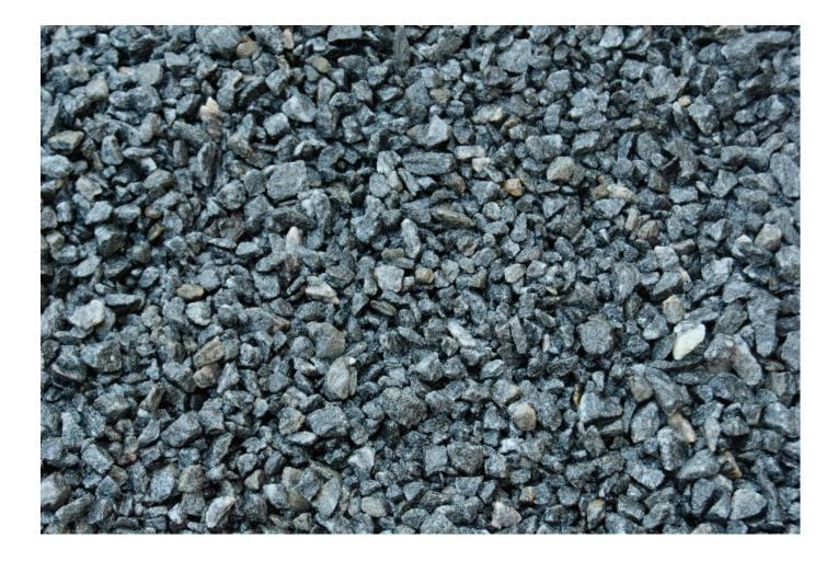
Proposed material: Crushed granite
