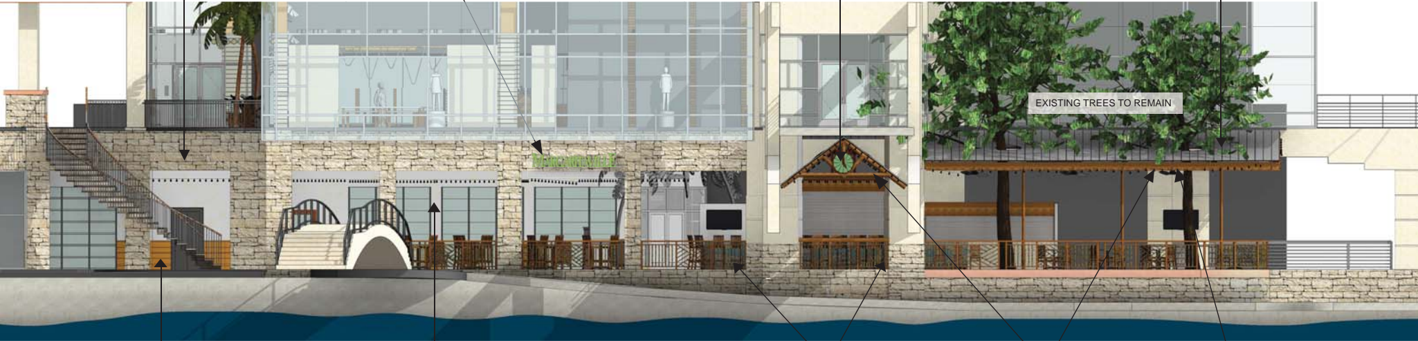
THEME PAINT-SIMULATED CONCRETE WITH JOINT LINES, RUST AND AGE STAINS
