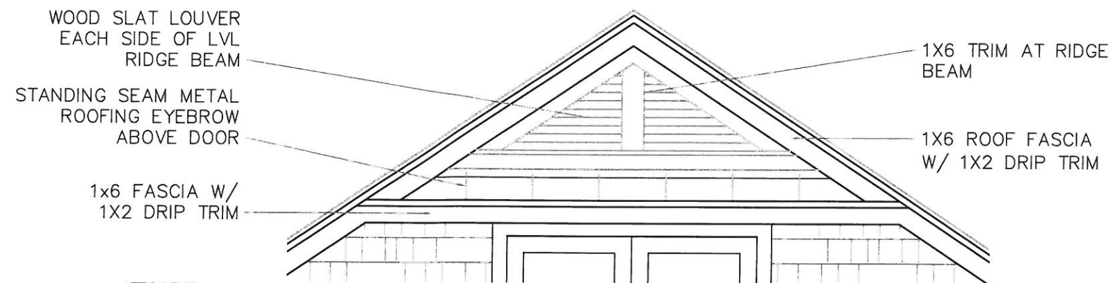
(B) GABLE VENT ELEVATION - Typical Front & Rear Elevation 3/4" = 1'-0"
