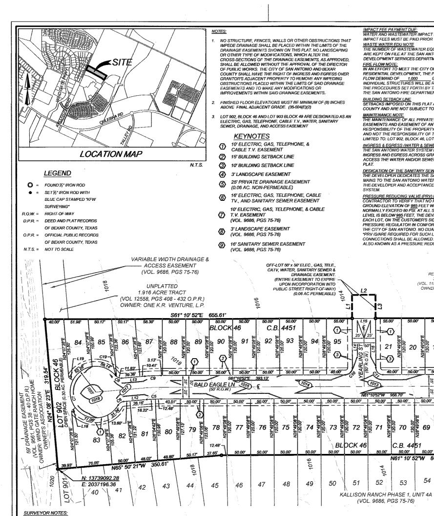
1/2" DIAMETER REBAR WITH A BLUE PLASTIC CAP STAMPED "KFW SURVEYING" SET AT ALL CORNERS UNLESS NOTED OTHERWISE
