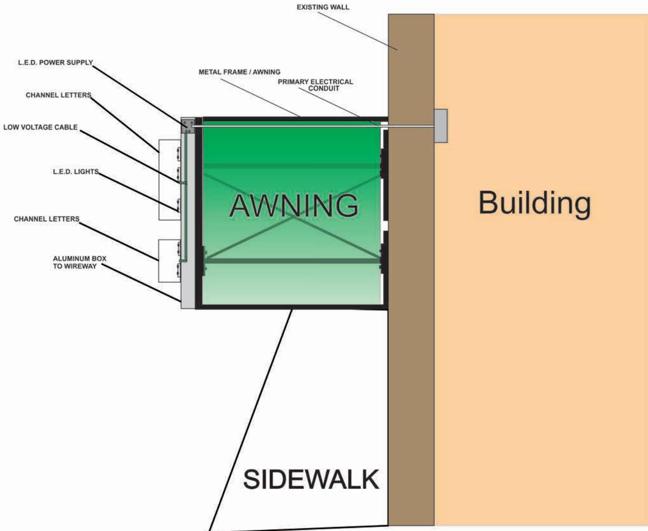
The awning has a metal frame attached to the wall and we have reviewed the frame and its sufficiently strong to hold the channel letters too.
