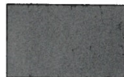
Weathered Galvalume SR=.30 E=.82
