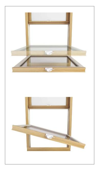
Next, tilt the top sash using the same technique described in the previous section. When the sash is in a horizontal position, lift both sides upward 2"-3" (51-76 mm) raising pivot pins out of the clutch. Finally rotate the sash until the pivot pins clear the jambs and remove the top sash from the frame.
