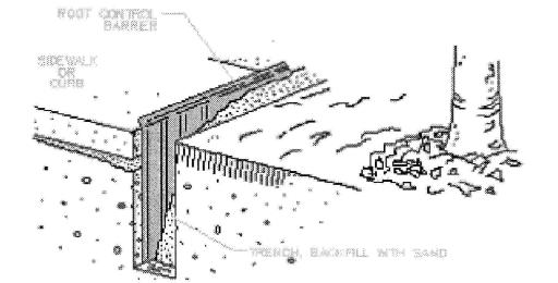
A VERTICAL UNDERGROUND BARRIER WILL HELP KEEP TREE ROOTS FROM DAMAGING CONCRETE AS
