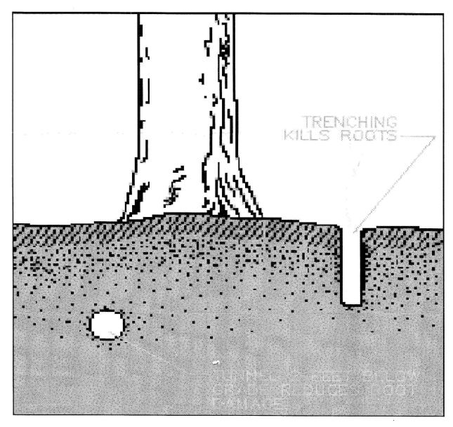
PROTECTS ROOTS FROM DAMAGE WHEN LAYING UTILITY LINES BY TUNNELING RATHER THAN
