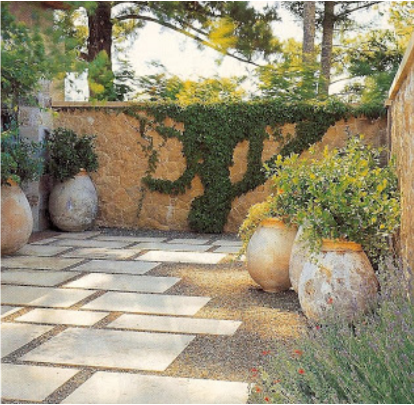
04 2 FT. X 4 FT. PATIO STONE IN DG -MORTAR SET BASE
