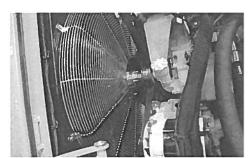
**OPERATING EFFICIENCY.** With features such as a hydraulically driven variable flow and reversing Flexxaire cooling fan, the TG5000 is built with operating efficiency top of mind. The fan adjusts the pitch of the blades based on temperature, which can increase the power available to the mill for better processing efficiency.
