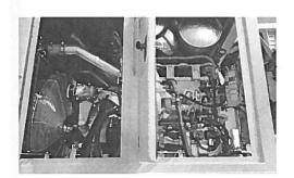
**ENGINE POWER.** The TG5000 is powered by a 540 hp (403 kW) Caterpillar C15 Tier 4 Final engine. A Tier 3 engine option is available for lesser-emission regulated countries.
