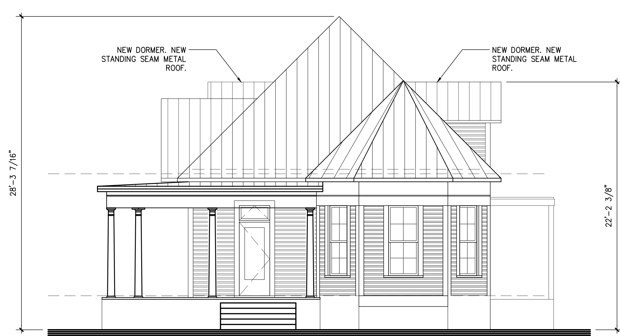
1 PROPOSED FRONT ELEVATION SCALE: 3/16"=1'-0"
