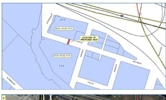
The sign will have an approximate 196 foot clearance and is to be located about 120 feet west of the Avenue A intersection.
