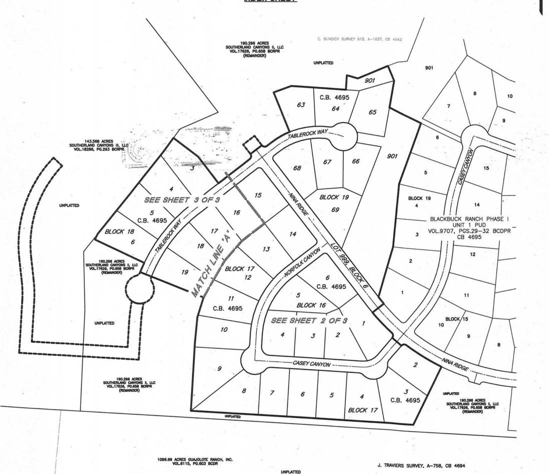
NO STRUCTURE, FENCES, WALLS OR OTHER OBSTRUCTIONS THAT IMPEDE DRAINAGE SHALL BE PLACED WITHIN THE LIMITS OF THE DRAINAGE EASEMENTS SHOWN ON THIS PLAT
