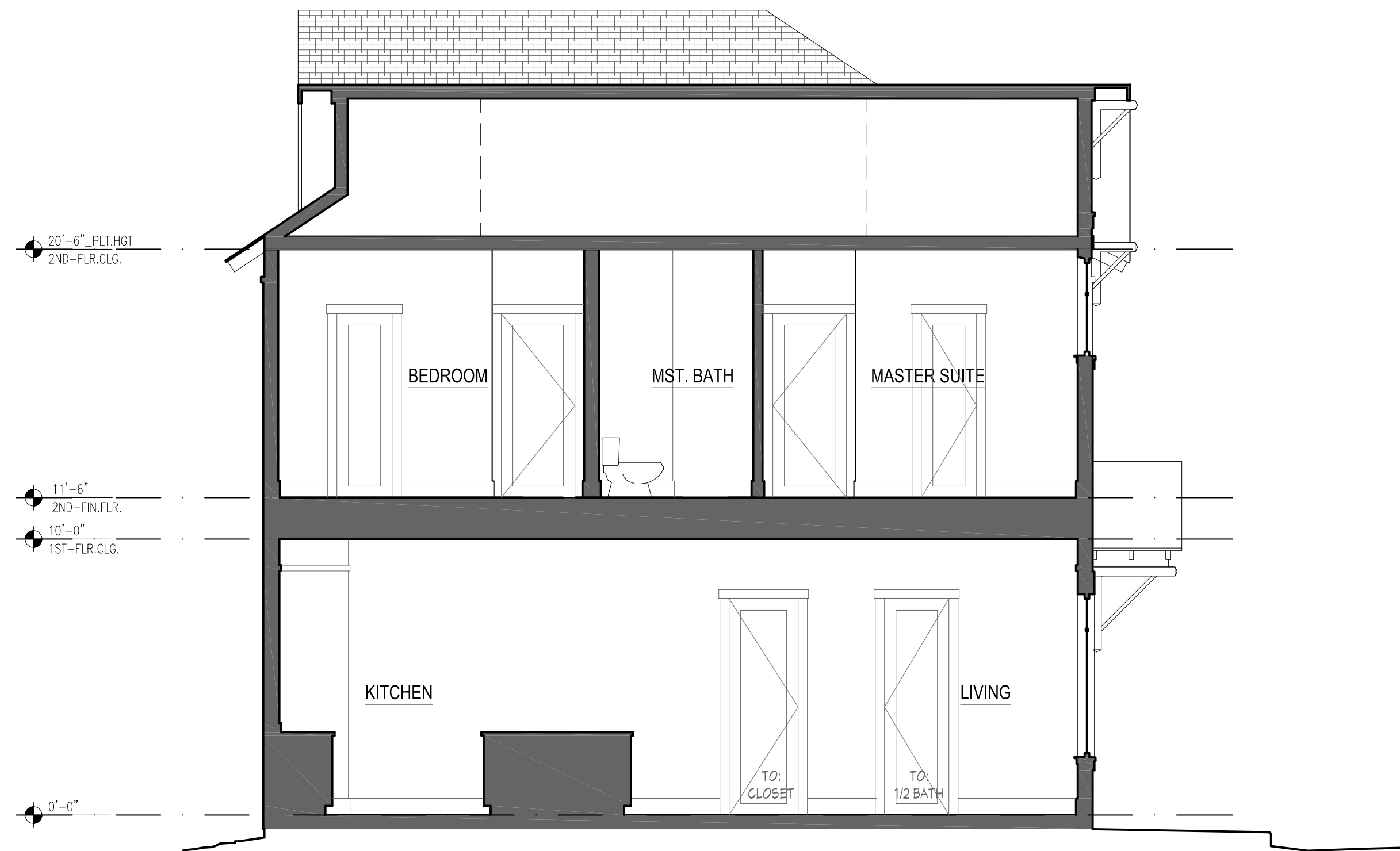
4 BUILDING SECTION SCALE: 1/4" = 1'-0"
