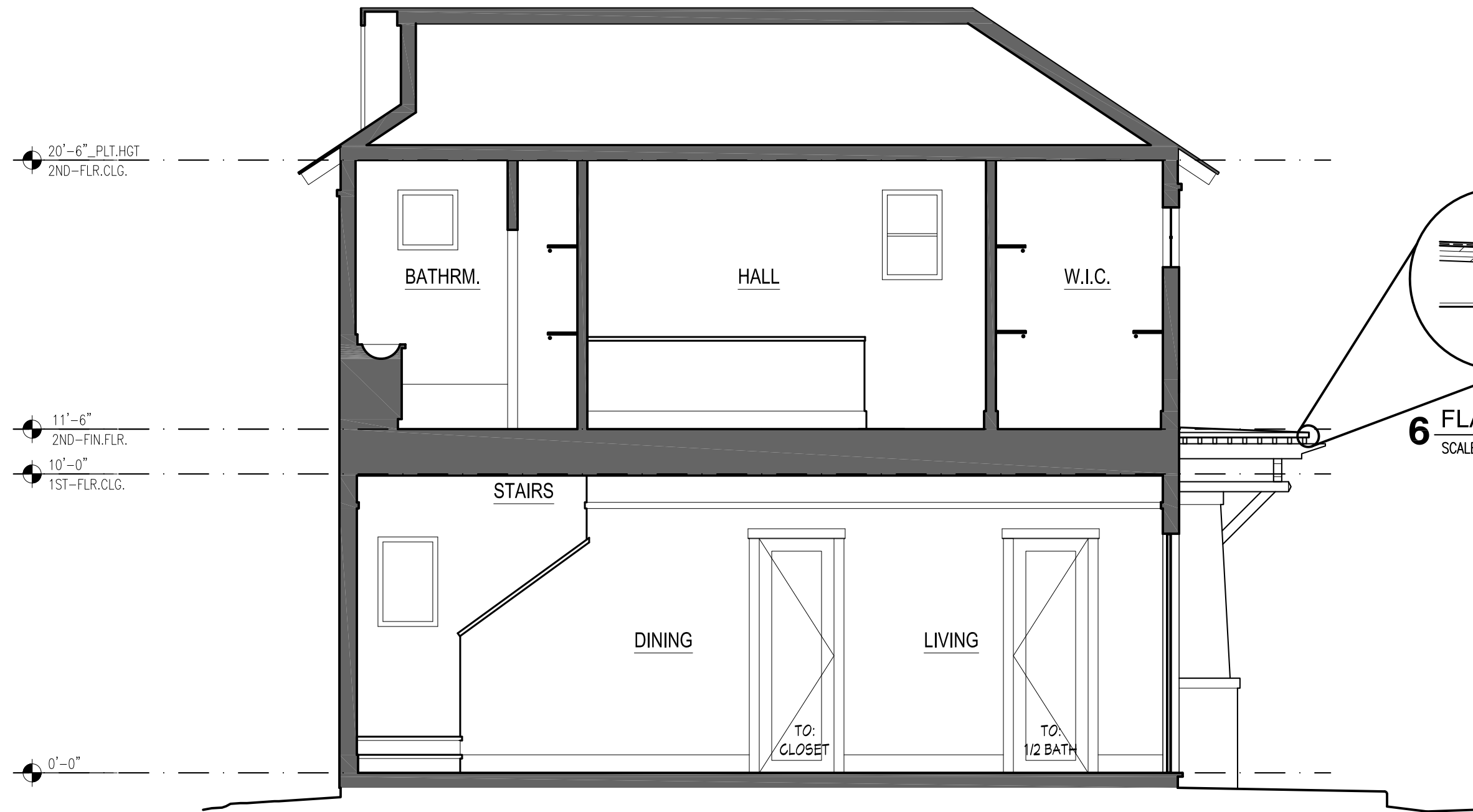
2 BUILDING SECTION SCALE: 1/4" = 1'-0"
