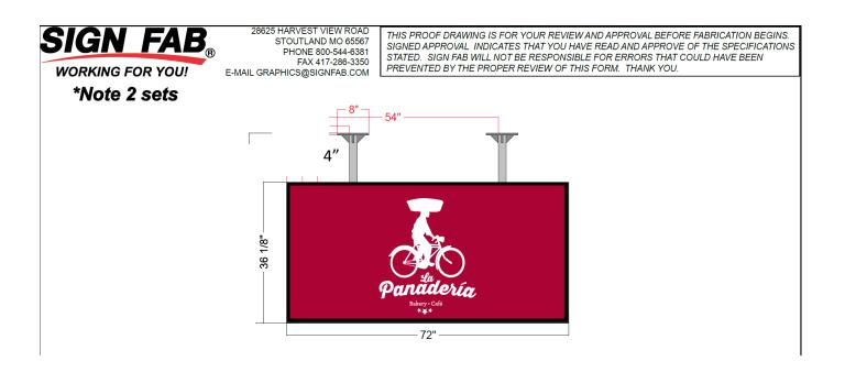
Specs: Two sets welded D/F cabinet w/ plex faces, aluminum trim & leds, square tube mounting arms & plates - self contained.
