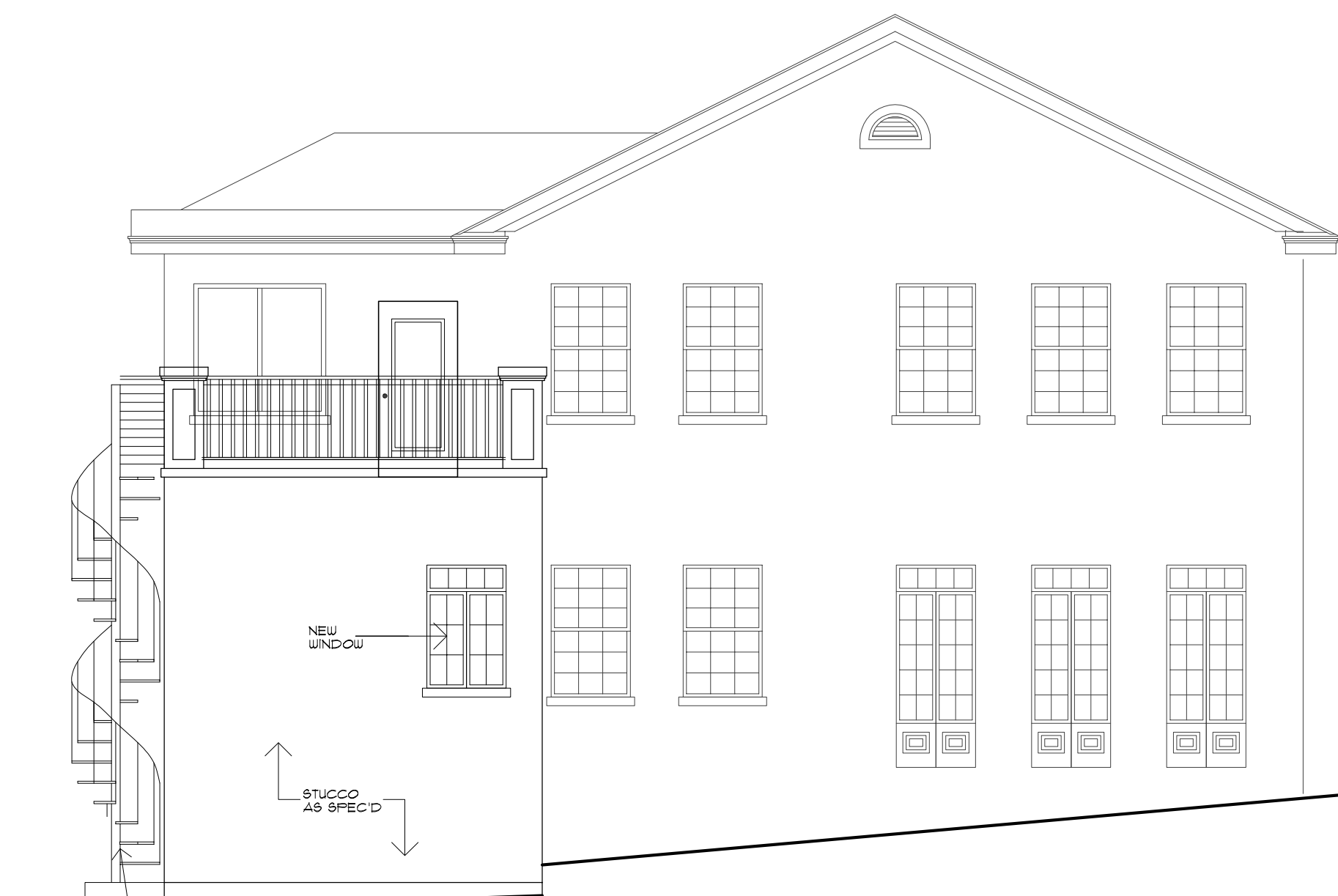
PROPOSED LEFT ELEVATION SCALE: 3/16" = 1'-0"
