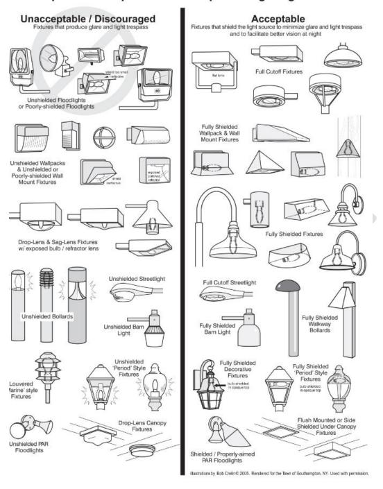
B. For lighting horizontal tasks such as roadways, sidewalks, entrances and parking areas, fixtures must meet "full cutoff" criteria (no light output emitted above ninety (90) degrees at any lateral angle around the fixture).
