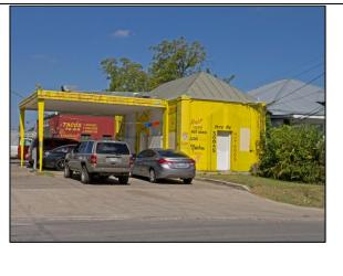
This filling station operated under the Humble brand through the 1960s. The structure has a rectangular footprint. The canopy supports are tapered, likely modified from the original piers. The roof of the structure is a hipped, standing seam metal roof and the canopy has a flat roof. The interior, however, still has a number of original details intact, including the mirror and tile on the bathroom floor and walls.
