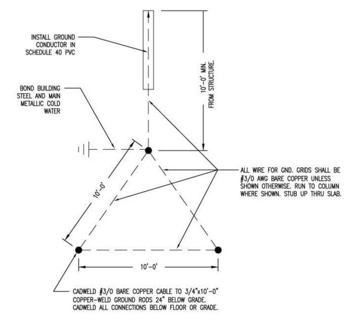
NOTE: PROVIDE A COMPLETE GROUNDING SYSTEM MEETING ALL REQUIREMENTS OF NEC ARTICLE 250.52 (A1) THRU (A6) AND 250.104 (A) THRU (C).
