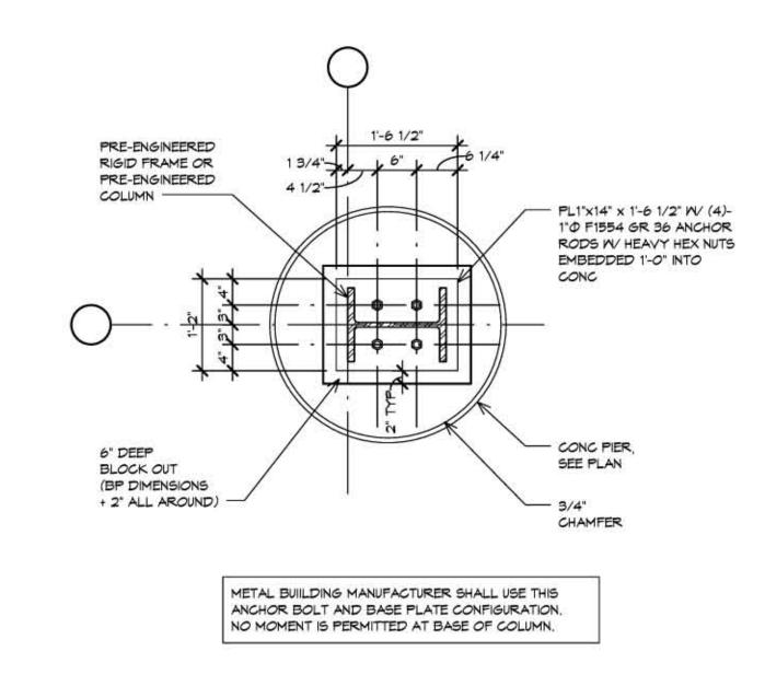
2 PLAN VIEW AT RIGID FRAME COLUMN BASE SCALE: 3/4" = 1'-0"
