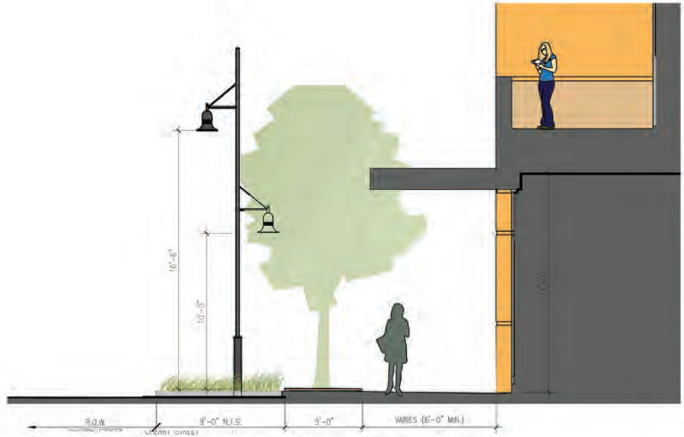
3 SIDEWALK SECTION (CHERRY ST.) SCALE: 1/4"=1'-0"
