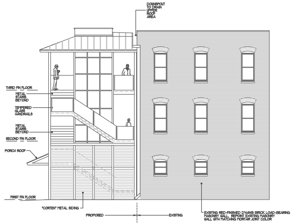
A-3.1.02 NORTH ELEVATION SCALE: 1/4" = 1'-0"
