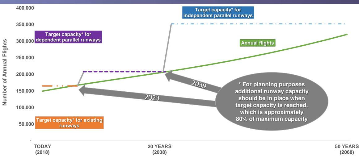
Dependent parallel runways are closely spaced (700 feet to 2,500 feet from an existing runway) and independent parallel runways are widely spaced (separated by at least 3,000 feet).
