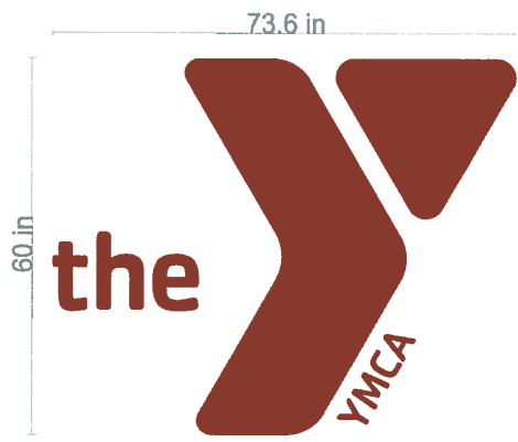
1/4" Flat-Cut Aluminum painted PMS 1685C Stud Mounted
