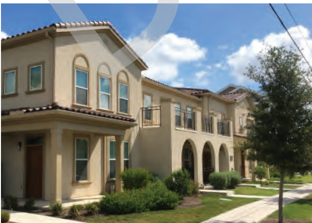
Photo 3.11 - Utilize offsets or architectural elements such as porches to create divisions in the wall plane.
