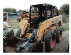
Equipped with:Solid Tires<br/>Grapple Debris Bucket<br/>Dirt Bucket<br/>Cyclone Concrete BreakerAdvantages:Has ability to get into small areas and handle<br/>debris. Solid tires increase productivity by no down-time due<br/>to flats. Interchangeable attachments allow more diverse<br/>production from one mobilization.Note:We currently have 4 of these units in our fleet.
