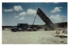
Equipped With: 30 CY End-Dump Debris Trailers 40 CY End-Dump Debris Trailers 50 CY End-Dump Debris Trailers
