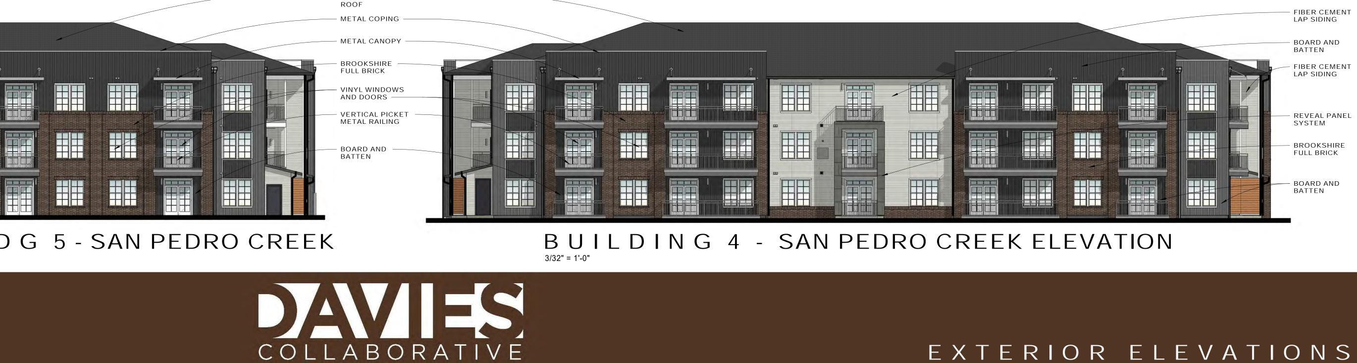
METAL COPING VINYL WINDOW REVEAL PANEL SYSTEM BOARD AND BATTEN FIBER CEMENT LAP SIDING
