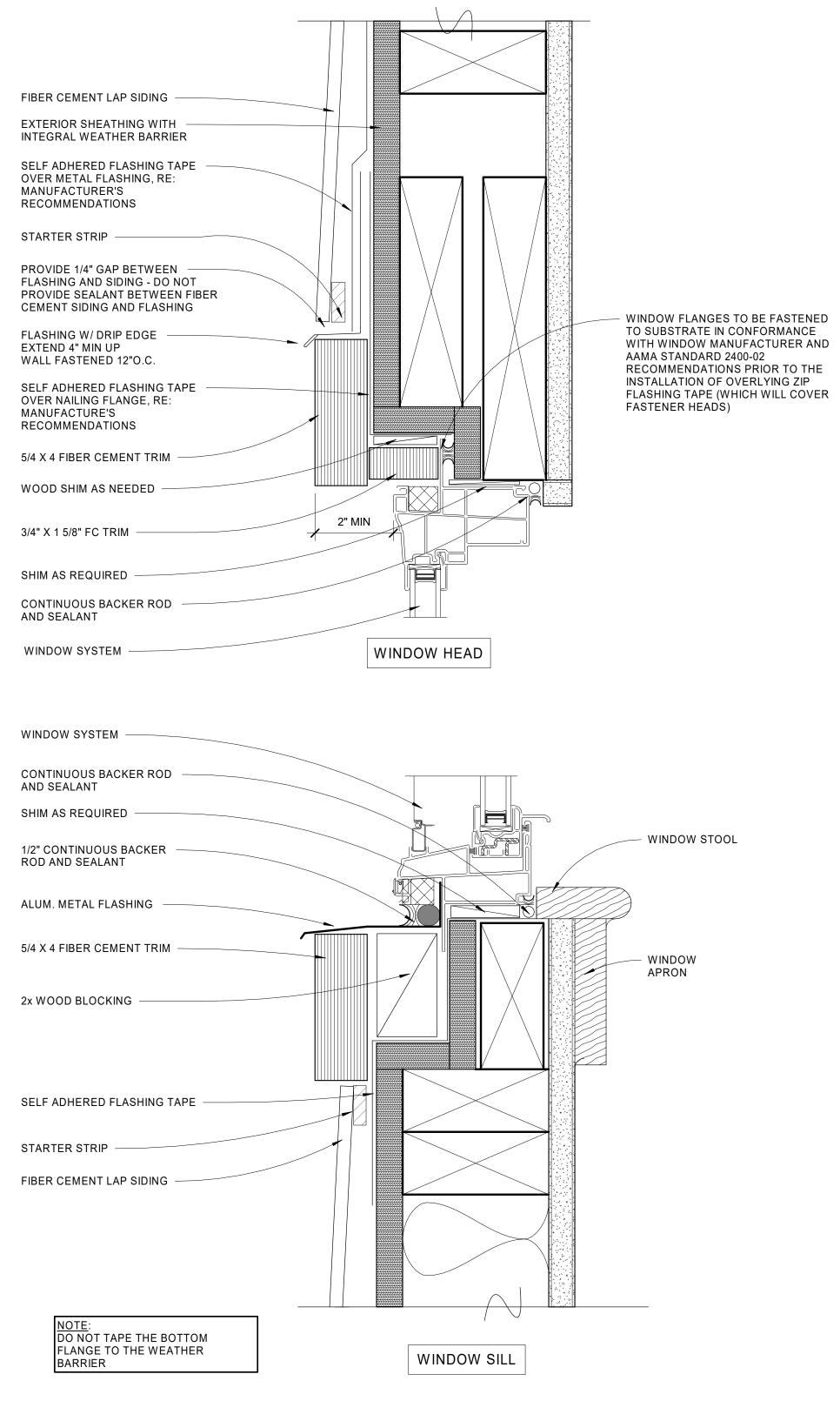
Window Details - HDRC Fiber Cement Siding, Woodtone Lap Siding and Board and  $3 \frac{\text{Batten Siding}}{6" = 1'-0"}$
