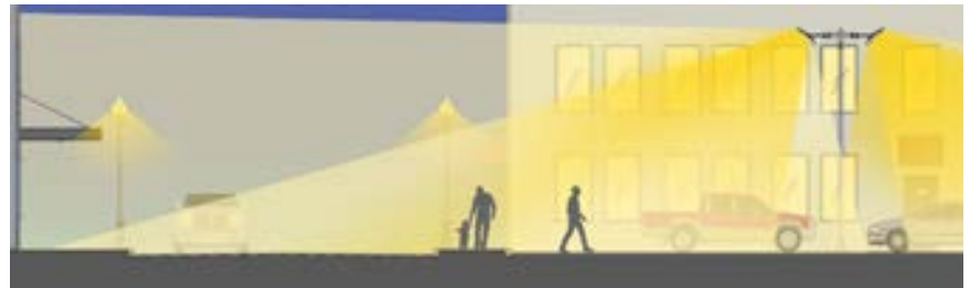
Nuisance glare from tilt-up style surface parking lot lighting can cause problems for both vehicular and pedestrian users.
