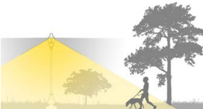
Retrofit and new fixtures that obscure the source and use a cutoff optic system reduce glare as well as greatly minimize uplight.
