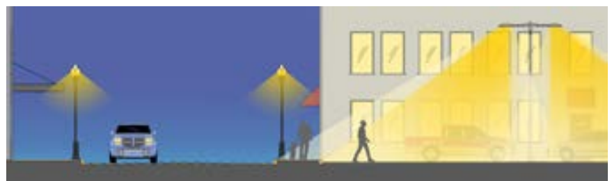
The use of luminaires with a full cut-off optic system will reduce glare, spill light, light trespass, and direct upward light.
