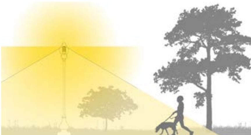
Traditional refractor ‘acorn’ style globe luminaires that utilize non-shielded sources creating both glare and excessive uplighting.
