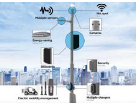
Integrated light pole and components
