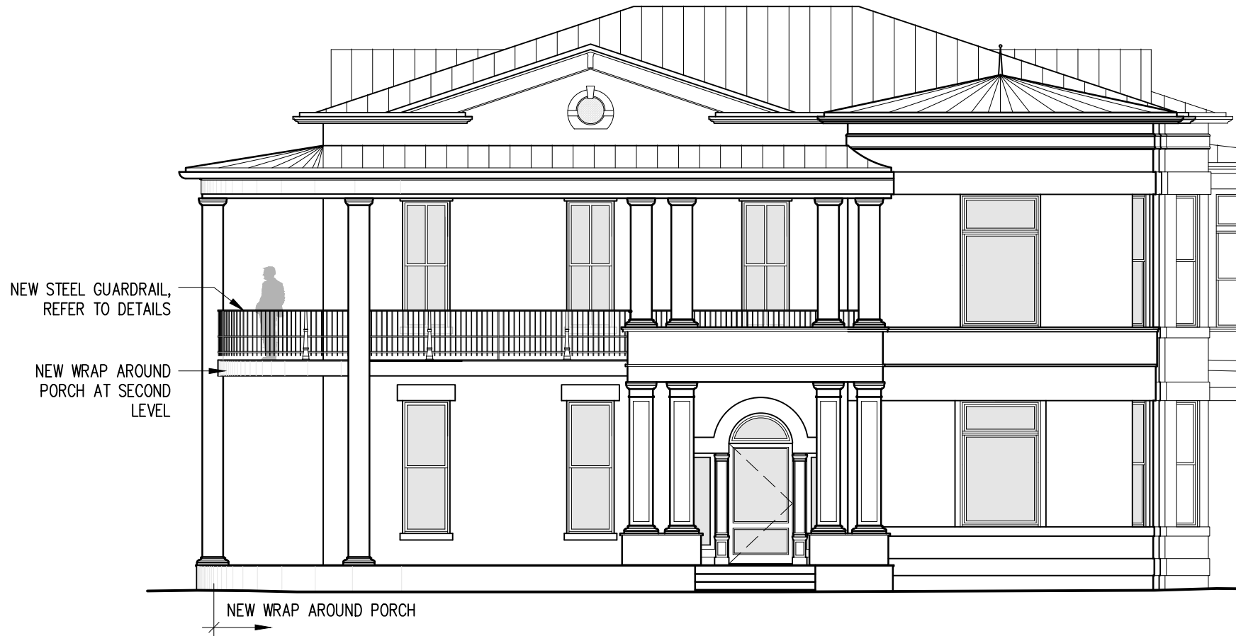
PARTIAL ELEVATION: SECOND LEVEL PORCH SCALE: 1/8" = 1'-0"
