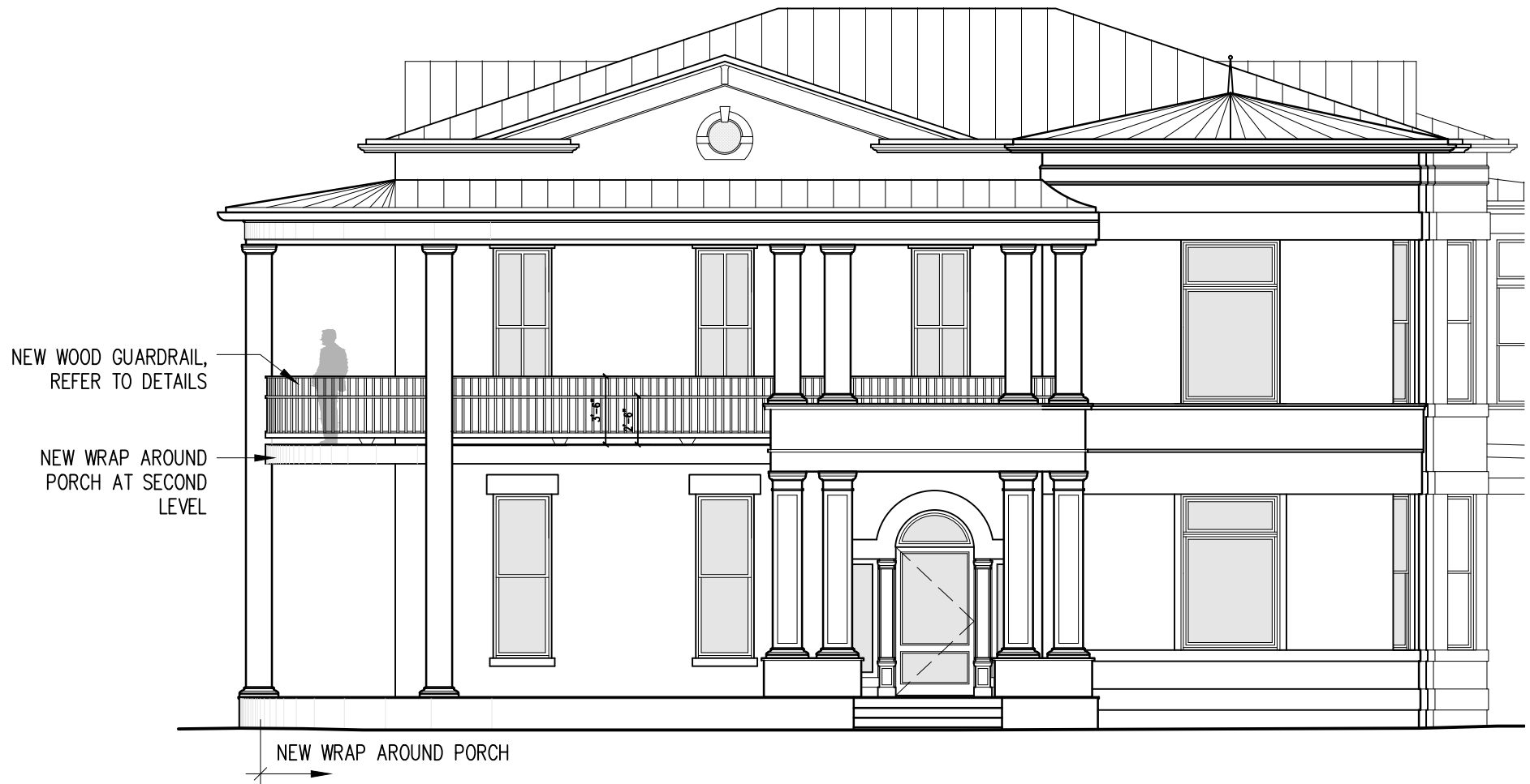
PARTIAL ELEVATION: SECOND LEVEL PORCH SCALE: 1/8" = 1'-0"
