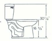
THIS FIXTURE QUALIFIES ACCORDING TO ASME TEST PROCEDURES AS A HIGH EFFICIENCY WATER CLOSET WITH AN AVERAGE CONSUMPTION OF 1.28 gpf (4.8 Lpf) OR LESS.
