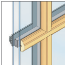
SIMULATED-DIVIDED-LIGHT WITH SPACER 7/8"
