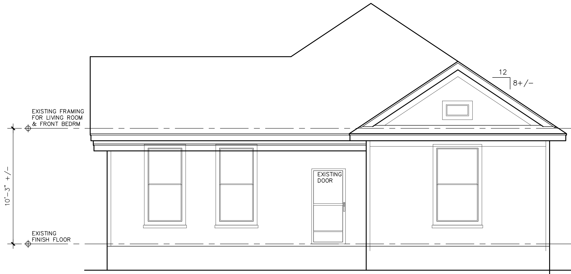
EXISTING FRONT ELEVATION SCALE: 1/4" = 1'-0"
