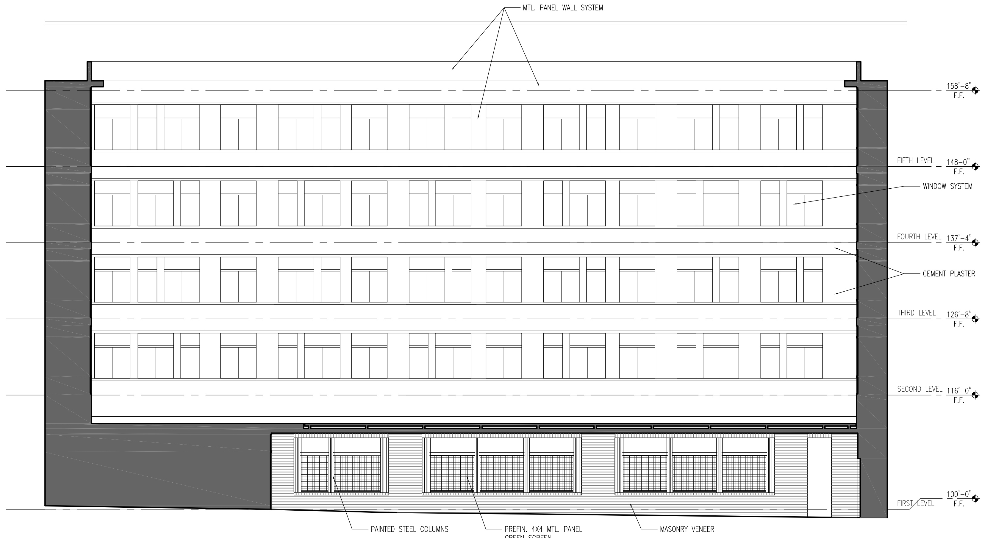
2 COURTYARD ELEVATION SCALE: 1/8"=1'-0"
