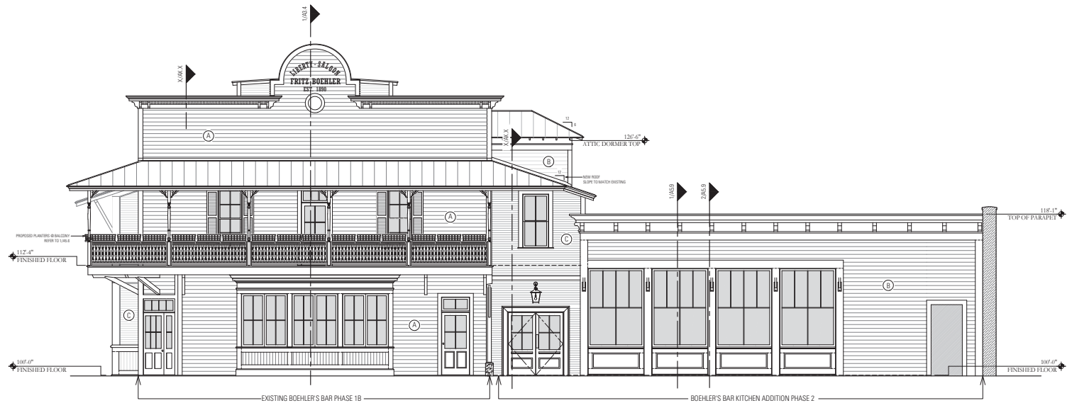
2 Boehler's Elevation - East - Without Stair & Awning Scale: 1/4"=1'-0"
