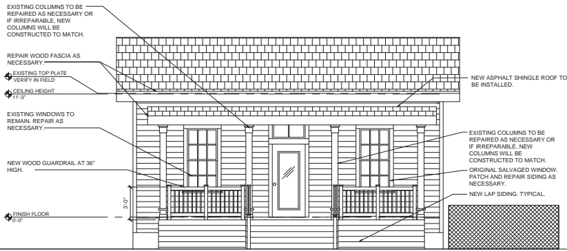
1 SOUTH ELEVATION Scale: 3/16" = 1'-0"
