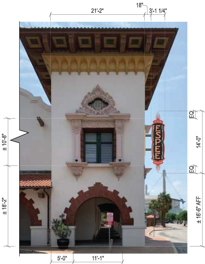
Main Building Blade Sign Elevations Scale: 3/32" = 1'-0"
