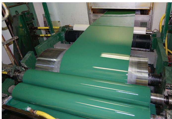
Berridge owns and operates its own modern continuous coil coating line in San Antonio, Texas, painting both 48" and 42" wide master coils.
