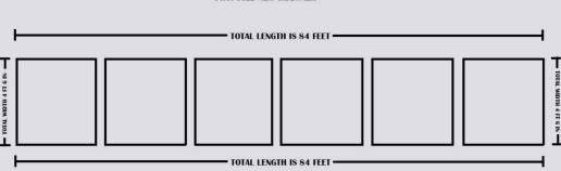
NOTE: THICKNESS OF CONCRETE WILL BE 5 INCH REBAR WILL BE 3/8 THICK PROPOSED NEW SIDEWALK
