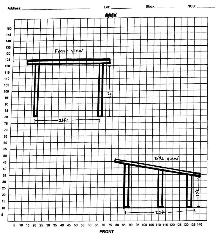
The materials for this project will consist of treated pine stained and cut to match the existing patio cover (see attached picture). The carport will consist of Six 4x4 posts, 2x8 beams, 2x6 rafters and 1x4 planks. The roof will be a standing seam metal.
