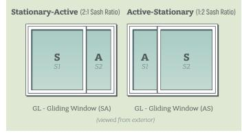
Two sash in one frame with a a 2:1 or 1:2 sash ratio. A = The active inboard sash operates
